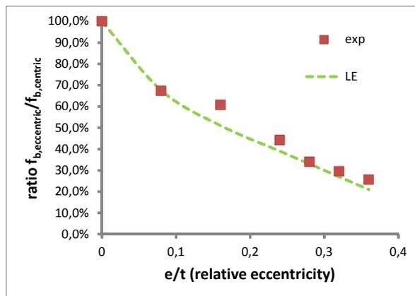
**Figure 2 Capacity reduction factor for masonry with Perinsul HL thermal break unit**
