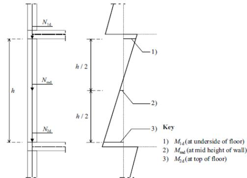
**Figure 1 Bending moments in vertically loaded masonry wall**
